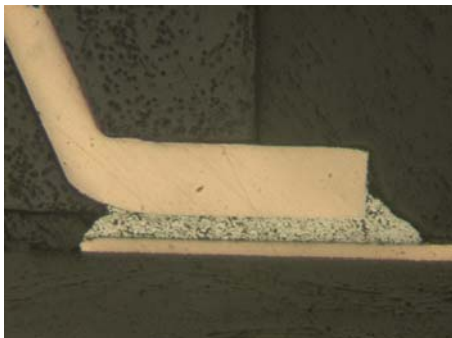
Figure 9: Cross-section of the DFL package lead's solder joint.
