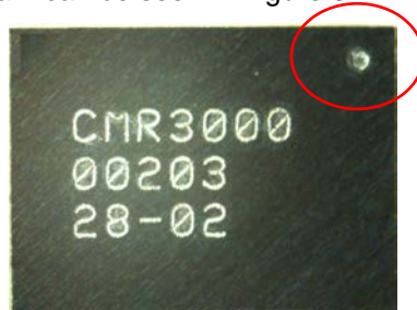
Figure 3. Pin 1 index mark on top of CMR3000.
