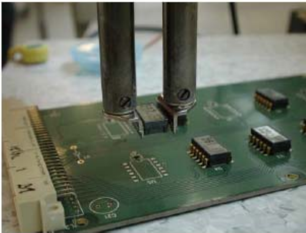
Figure 14. Immediately after solder melting, component is lifted.
